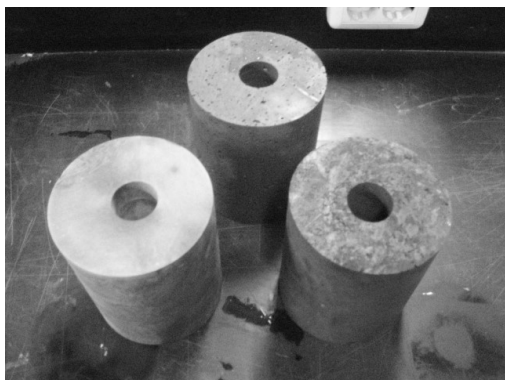
Fig. 5. Hollow specimens for permeability test
